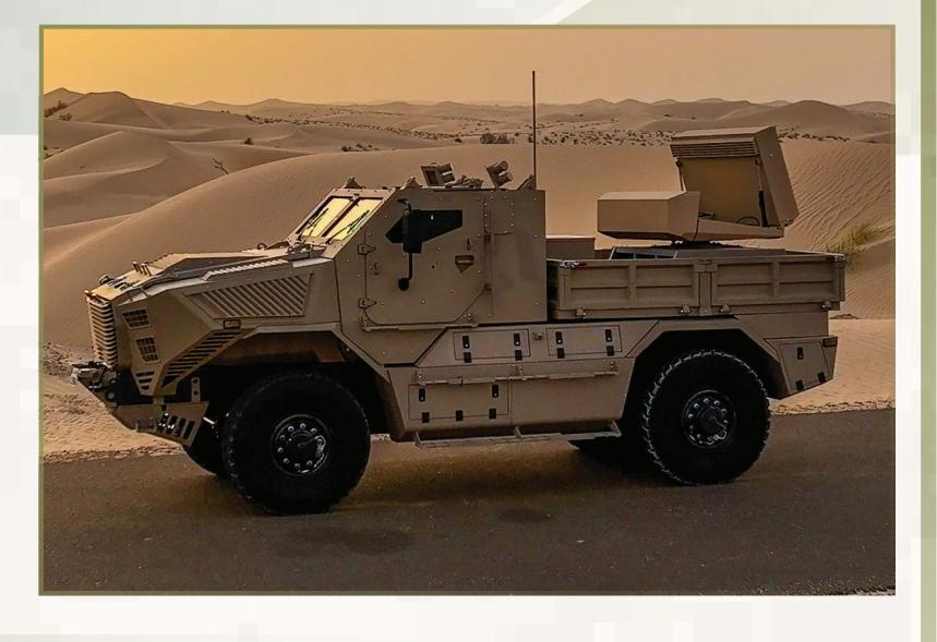
GVW = 16.5 ton, curb weight = 12.4 ton, payload = 4.1 ton.
